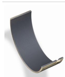
Polymer coated lead free silver based overlay material. used for applications that require a bearing to withstand extreme loads, high pressure and metalto-metal contact due to minimal oil film thickness.
