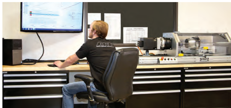
ARP's computer-controlled torque-tension machine can apply a given torque or torque-angle to a fastener and measure the clamp load. Through test cycles, it is possible to chart the clamp load scatter with various fasteners and lubricants.
