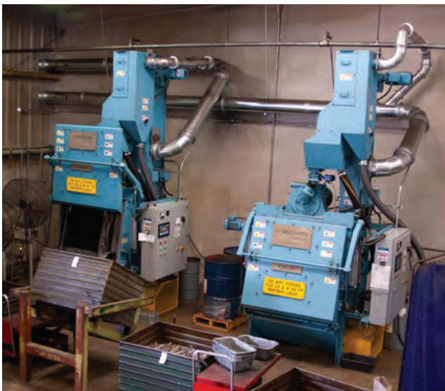
Fasteners are shot-peened to improve fatigue life.
