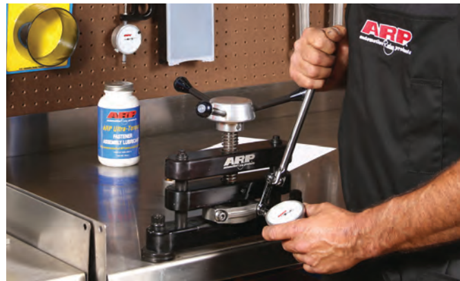
A rod bolt stretch gauge is one of the most important tools a serious engine builder can own. It's valuable in properly setting up a rod for resizing, obtaining the proper clamp load when installed. See page 135 for more information.
